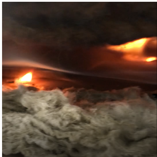
Figure A.7: Bitumen dropping on to the top plate
