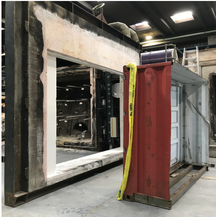
(a) Door section before mounting in to the test frame
