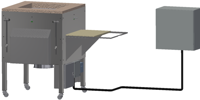
Figure A.1: The Mobile Furnace
