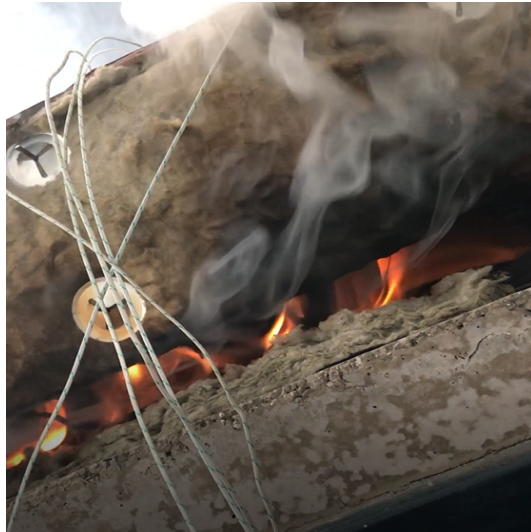
Figure A.5: Flames inside the cavity
