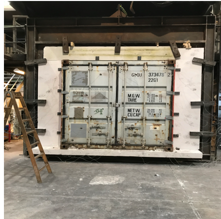
(b) Door section after being mounted in test frame
