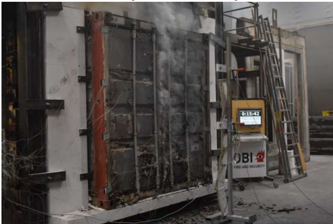
A bit after 14 minutes smoke starts again and at 17 minutes sealing catches fire
